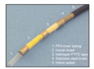
The table with technical data below shows specifications for the Highflex hoses. We recommend the Highflex hose when the demands for pressure and flexibility are extremely high. The hose is designed with an innertube of PFA or PTFE<sup>1</sup>, a layer of Kevlar braid<sup>2</sup> which is separated by a PTFE<sup>3</sup> layer from the braid in stainless steel<sup>4</sup>, in order to avoid friction and finally an outer cover of Hytrel<sup>5</sup> for outer wear resistance.
